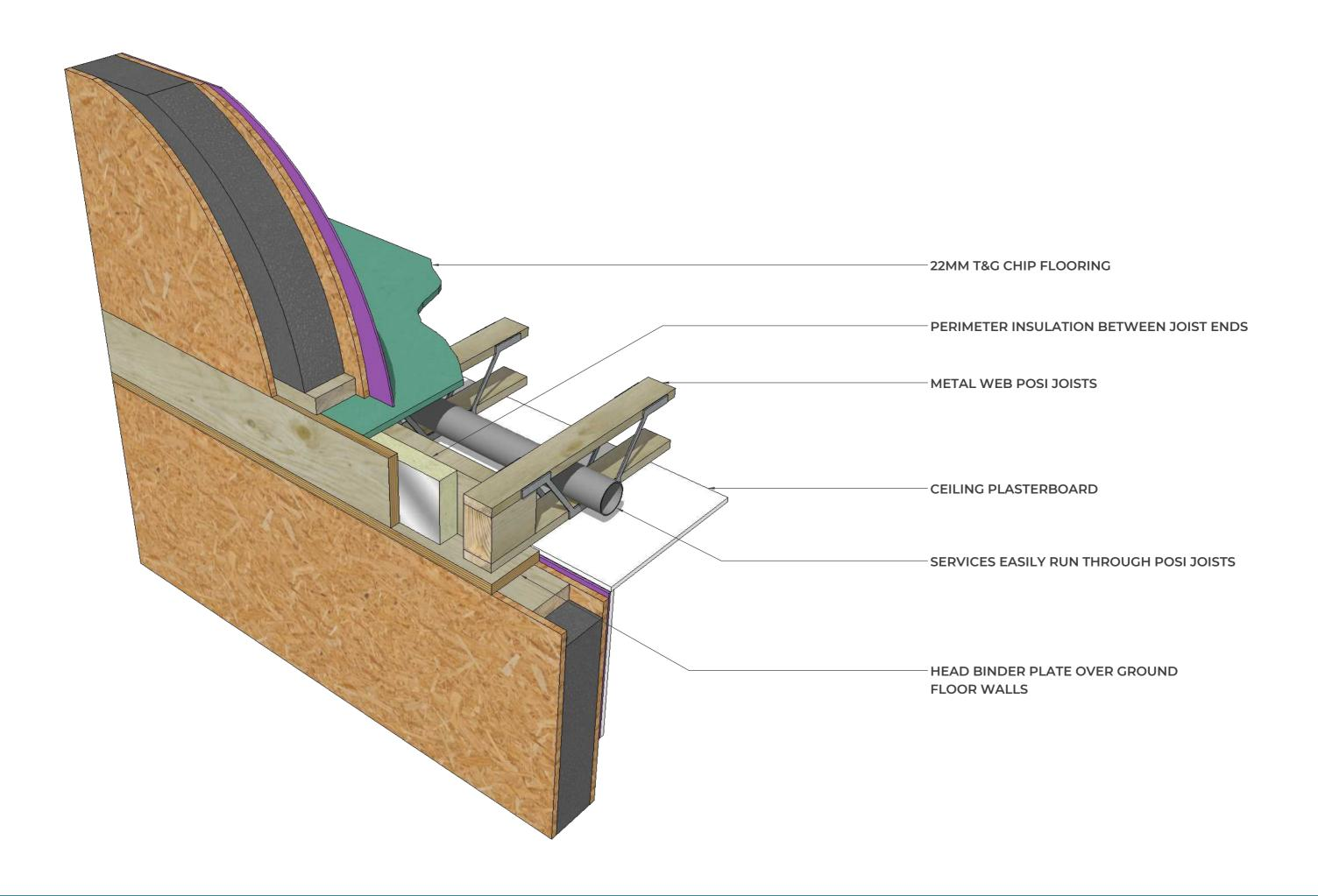
**POSI JOIST FLOOR FULLY SUPPORTED ON SIP WALLS**
